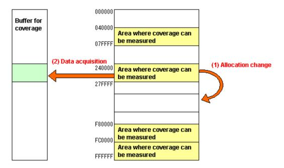
Figure 5.75 Schematic of coverage memory allocation change
